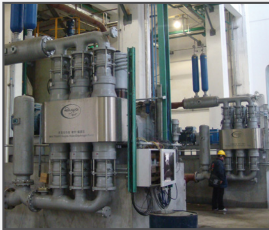
Triplex sets of FELUWA MULTISAFE® double hose-diaphragm process pumps with double ball valve configuration feeding coal slurry at high pressure into a gasifier.
